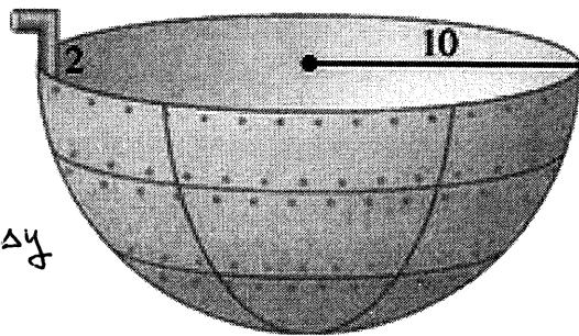
$$\begin{aligned} \text{Total Work} &= \int_0^{10} \pi \rho g (y+2)(100-y^2) dy = \pi \rho g \int_0^{10} (200 + 100y - 2y^2 - y^3) dy \\ &= \pi \rho g \left[ 200y + 50y^2 - \frac{2}{3}y^3 - \frac{1}{4}y^4 \right] \Big|_0^{10} = \pi \rho g \left[ 2000 + 5000 - \frac{2}{3}(1000) - 2500 \right] \\ &= 500\pi \rho g \left[ 4 + 10 - \frac{4}{3} - 5 \right] = 500\pi \rho g \left( \frac{23}{3} \right) = \frac{11500\pi \rho g}{3} \end{aligned}$$
