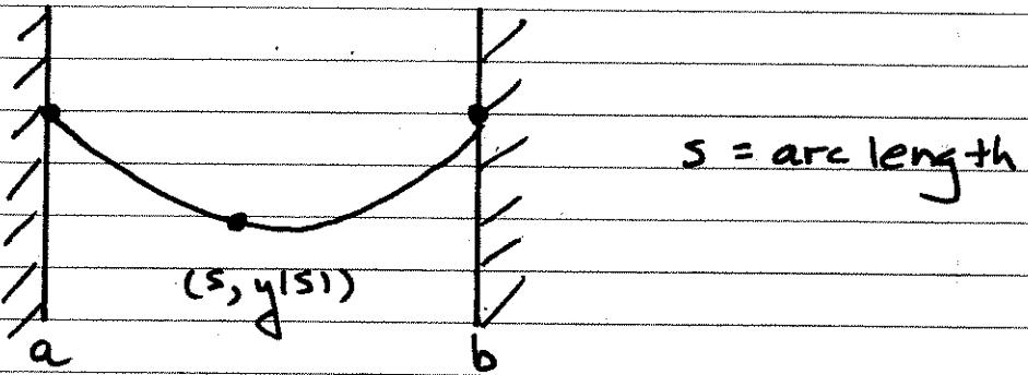
Cable of length  $L$  has a shape which minimizes the gravitational potential energy.
