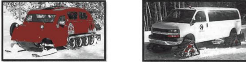
Figure 2: Examples of snow-coaches that were converted from street use for use on snow-roads.
